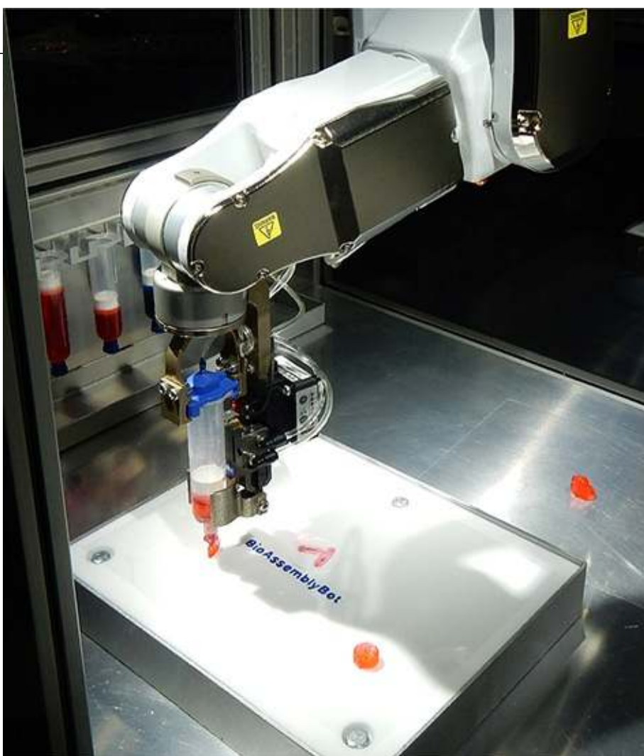
Figure 1-7 A printer making arteries with biomedical filament.
