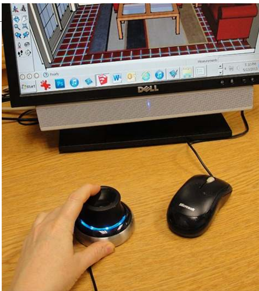
Figure 1-13 The Space Navigator mouse by Logitech is designed for the 3D environment. It can be used along with a traditional mouse.
