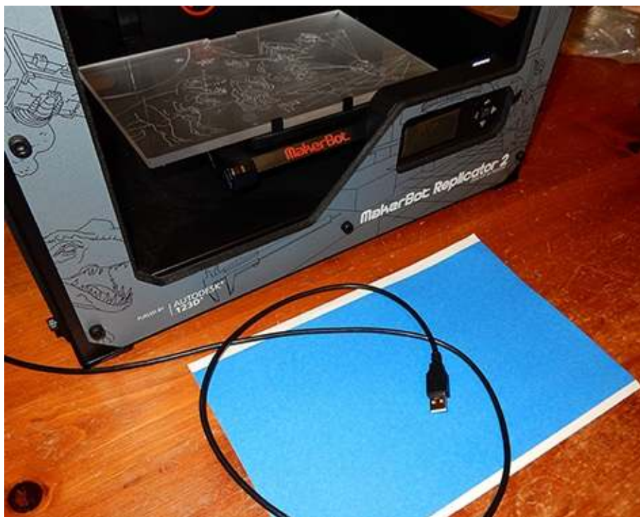
Figure 1-5 A 3D printer plugs into a computer USB port.
