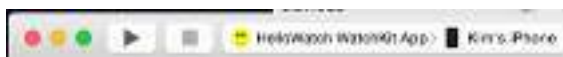
Figure 1-17. Choosing the scheme and target to run the example on your watch
